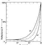
as a function of incident angle  $\theta$  (the angle to the normal) is given here for convenience. The graph is for the case of glass, but is only marginally different in the water case. It shows the reflectance for the two polarizations parallel and perpendicular with respect to the plane of incidence. The dashed curve is the average, or the effective reflectance for non-polarized light.
